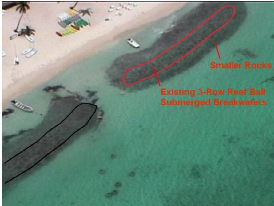
Figure 8. Delineation between the original Reef Ball breakwater and smaller rocks.
