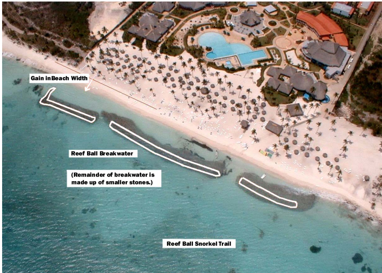
Figure 7. Delineation of the Original Reef Ball™ Breakwater and Small Rocks. Aerial photograph taken April 28, 2001.
