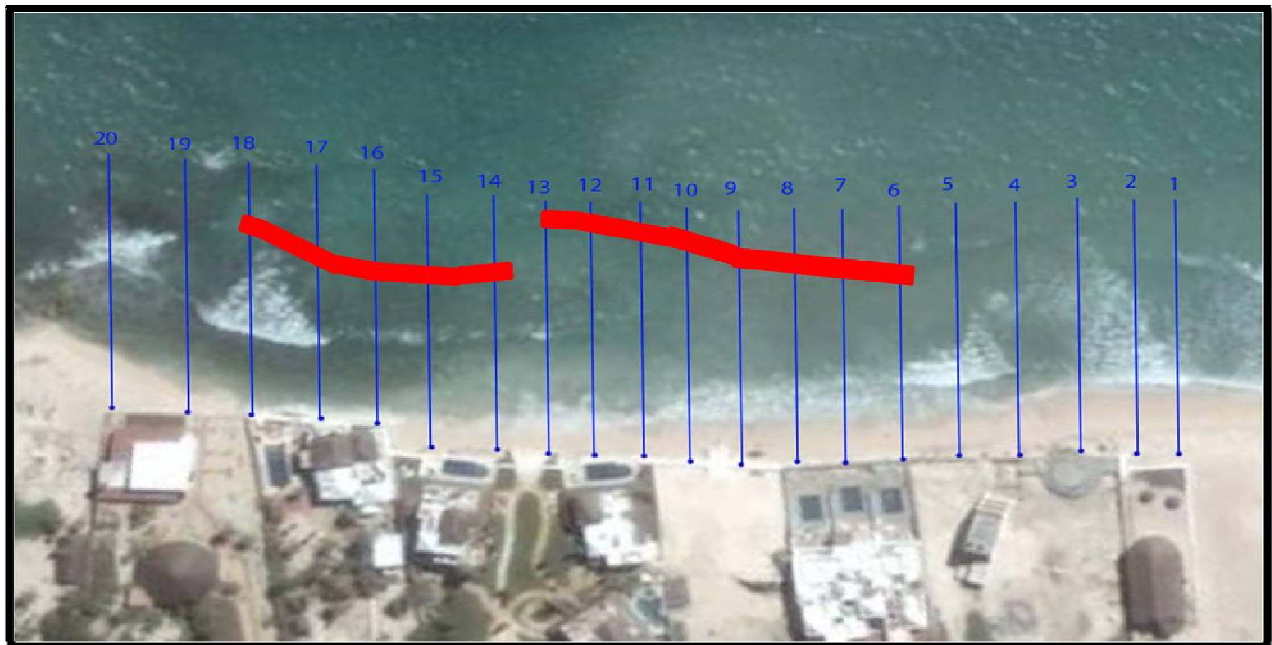
Figure 18. Plan View of Proposed Submerged Artificial Reef Breakwater
