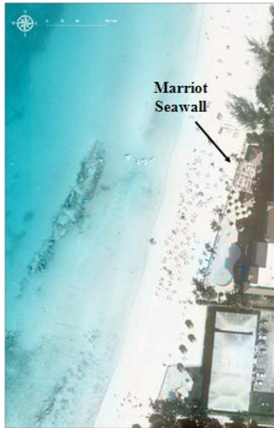
Figure 16. Aerial image from 1994 showing location of Marriott Seawall and width of beach in front of the seawall.
